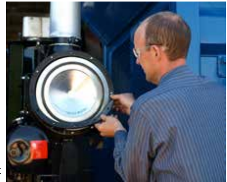
When servicing the EBB, make sure to replace the cover gasket when changing filters.
