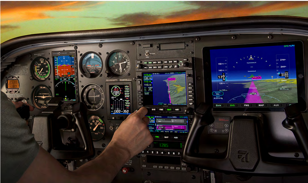
Cessna 206 - IFD550, IFD440, AMX240, AXP340 & IFD100 on iPad
