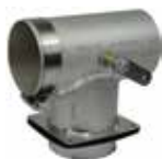
2 1/2" INLET & 2" OUTLET HOME-BUILDERS CABIN HEAT BOX This box is identical to the deluxe stainless steel cabin heat box, except that the inlet is 2 1/2" OD so that it can be used on larger heat muff applications where the builder is using 2 1/2" scat tubing. This box is currently being used on the MICCO certified aircraft. Weight is 7.2 ounces. P/N 08-04013 .....$218.95
